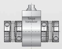
Smaller bore diameters at reduced torque capacities available upon request
